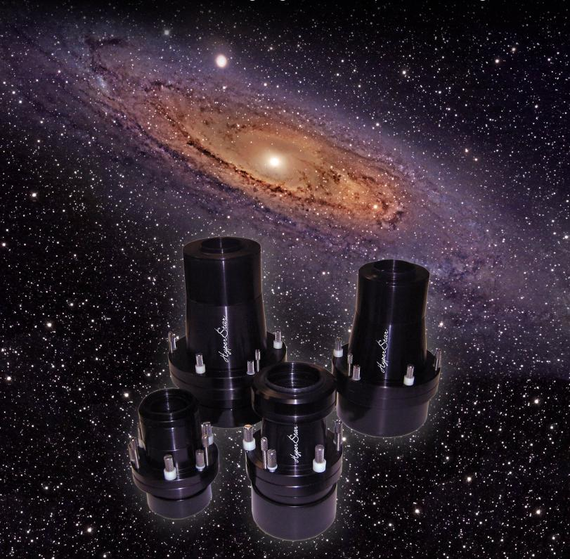
The HyperStar lens converts a standard Schmidt-Cassegrain telescope to a fast imaging system. The lens quickly and easily replaces the secondary mirror in the telescope, allowing a camera to be attached at the front of the telescope. The telescope is converted from an f/10 system to an ultra-fast f/2!
