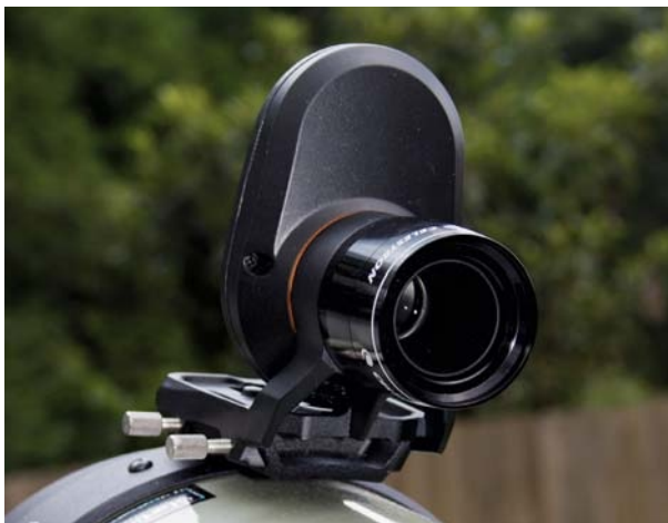
The Celestron StarSense camera takes the place of the standard 9x50-mm finder when used. This camera automates the Go To alignment process.
