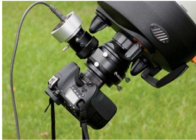
A DSLR is attached to the Celestron off-axis guider. The auto-guider camera is not part of the reviewed Celestron package.
