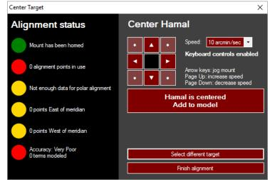
After one alignment star your CGX is minimally aligned. We recommend aligning to at least 4 stars for better goto accuracy, or ideally until all fields in the Alignment Status Window turn green.
