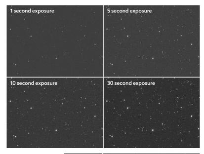
A A comparison of 1, 5 and 10 and 30 second exposures on a random star field in Gemini reveals how quickly the RASA-8 digs deep. The 1 second image records stars down to 15th magnitude while the 30 second exposure approaches mag. +18
