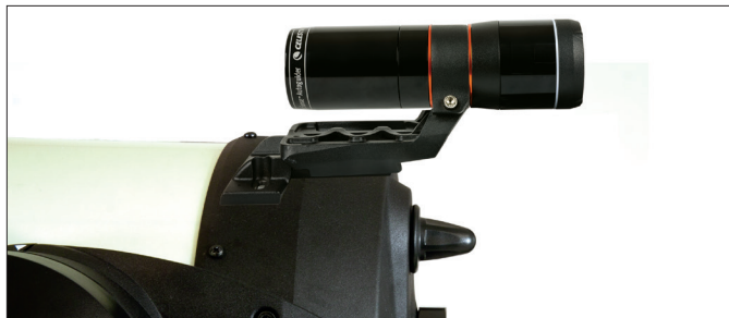
Fig. 5a: You'll need to install the base and large bracket backwards on a CPC 800 telescope.
